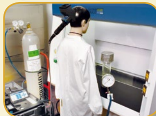
Tracer Gas (SF 6 ) Containment Test
